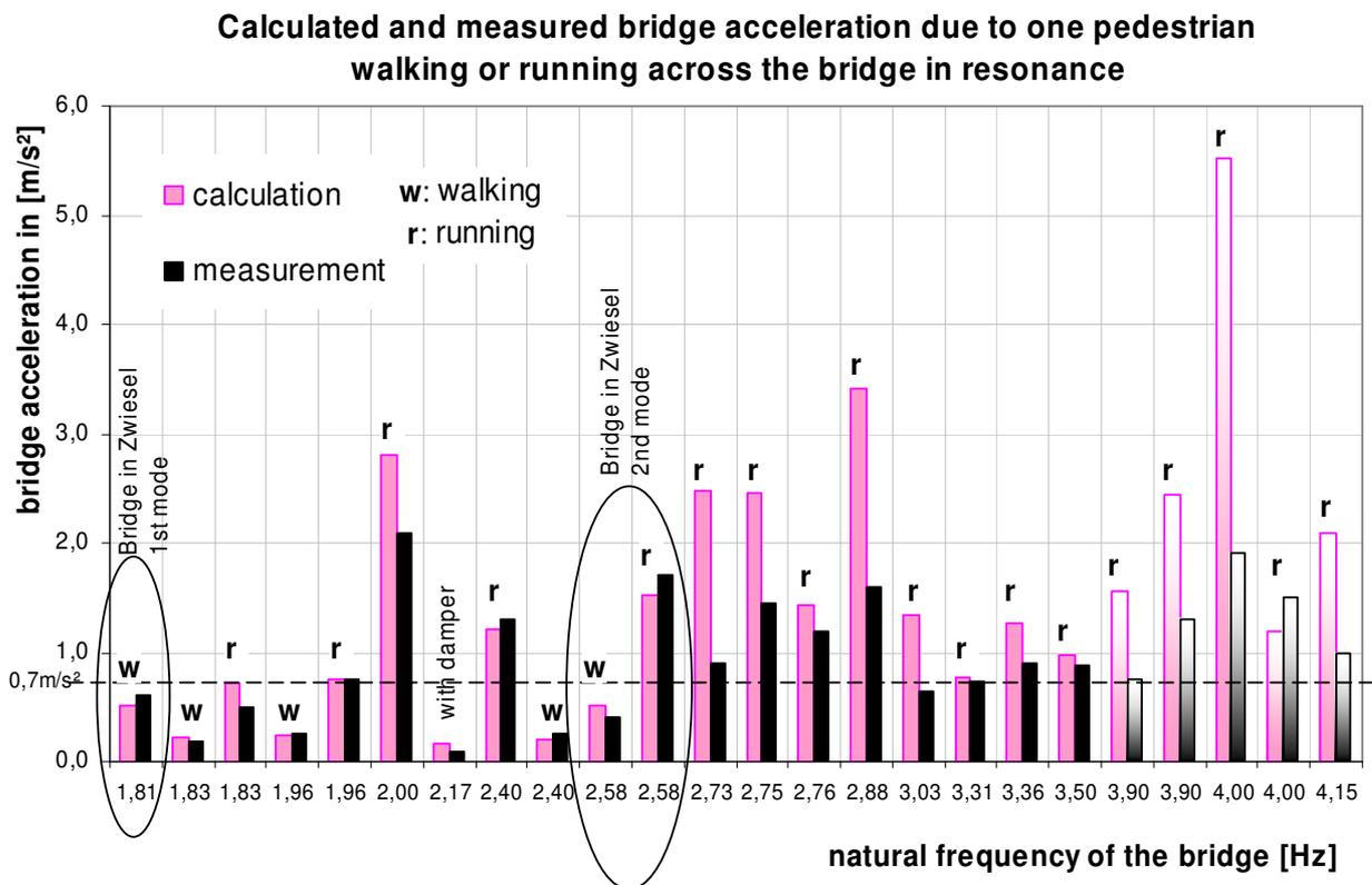
Figure 6: Comparison of calculated and measured bridge accelerations due to one pedestrian walking or running across the bridge in resonance
