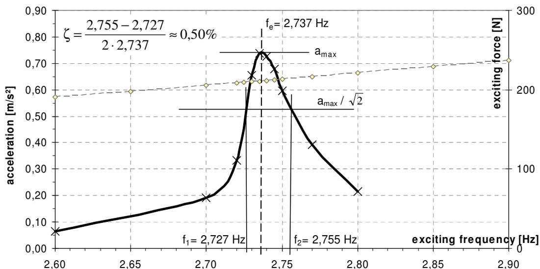
Figure 9b: Resonance curve (measured acceleration and exciting force) for a wooden footbridge in Oberesslingen.
