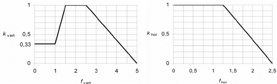
Figure 4a, b: Relationship between the vertical /horizontal natural frequency and the coefficient  $k_{\text{vert}}$  and  $k_{\text{hor}}$ , taken from [1]
