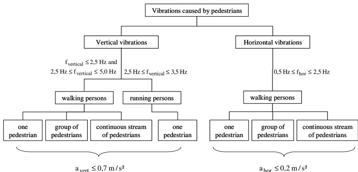
Figure 1: Verifications of bridge vibrations caused by pedestrians recommended in [1], [2], [3]
