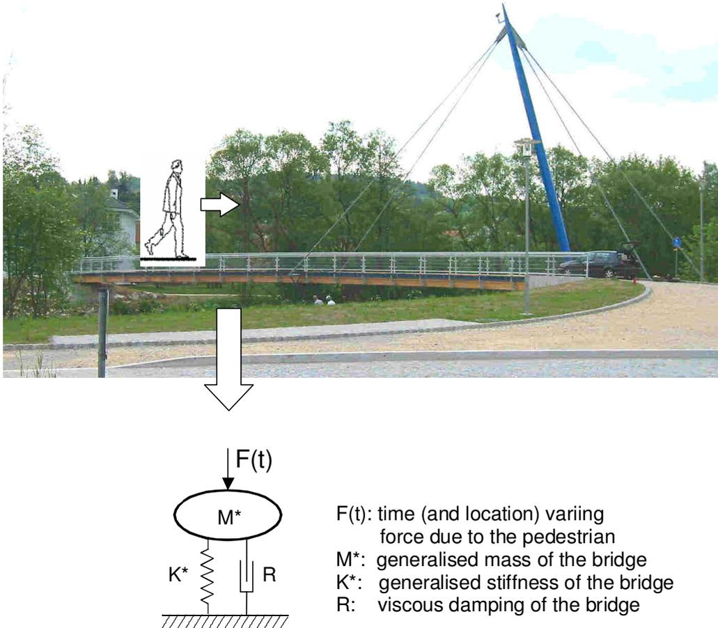
Figure 2: Footbridge in Zwiesel: Picture and dynamic model of the bridge incl. pedestrian
