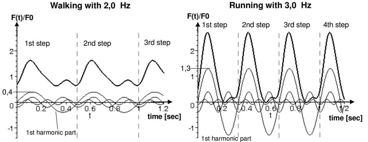
Figure 3: Graphs of the loads due to a walking and running pedestrian (total (thick line) and the first 3 harmonic parts (thin lines))
