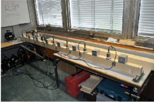
Figure 8: Beam B1 loaded with an additional mass
