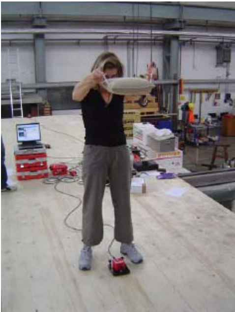
Figure 13: Test taker on CLT plate dropping a sand bag
