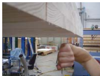
Figure 11: Excitation by punching with the fist
