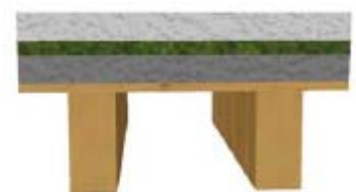
Figure 10: Heavy floor made of (from top): 60 mm anhydrite screed 30 mm foot fall sound-damping on 60 mm grit
