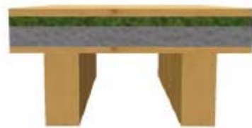
Figure 9: Light floor made of (from top): one layer OSB as a light screed 30 mm foot fall sound-damping on 60 mm grit
