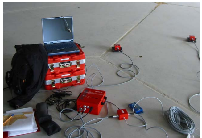
Figure 4: Measurement device with recorder (middle) and acceleration sensors (right)
